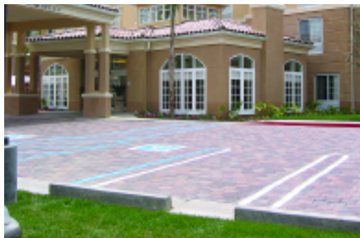
Figure 3. Curb cuts at this hotel parking lot in southern California allow overflow water to drain from the parking lot during flood conditions.
