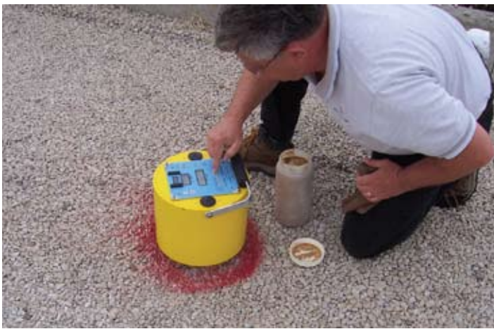
Figure 4. In contrast to a nuclear density gauge, the Geogauge device measures base stiffness which can indicate when compaction is complete. Unlike a nuclear density gauge, operating this device does not require certification.
