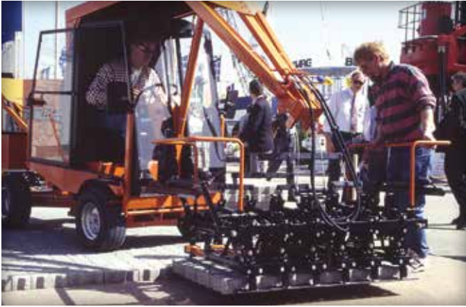
Figure 3. Motorized equipment with a mechanical clamp.
