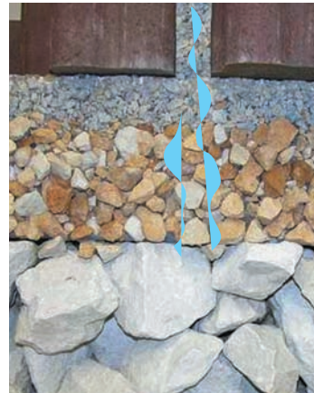
Permeable interlocking concrete pavement (PICP) with base and subbase for infiltration and storage
